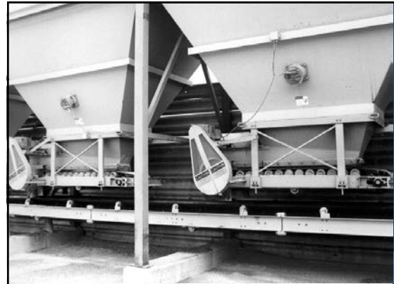
Electronically controlled variable speed belt conveyors at the individual feeders
